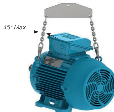
Figure 7 - Maximum resulting angle for motors with two or more lifting eyebolts
