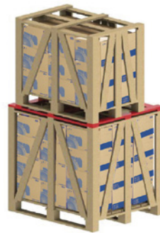
Figure 28 - Use of additional battens for stacking
