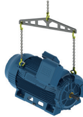
Figure 7 - Lifting with vertical chains.
