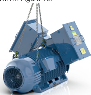
Figure 10 - Lifting of motors with two main terminal boxes.
