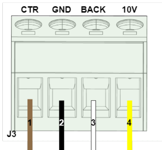
Figure 12 - Controller sequence connection.
