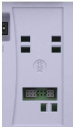
Figure 9 - XC3 bluetooth or ethernet accessory connector.
