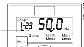
Illustration 7.7 Indicating Motor Direction
