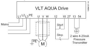
Figure 12.5 Wiring for Submersible Pump Application
