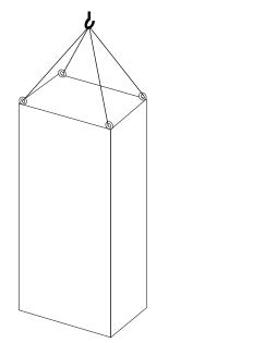
Figure 9.4 Recommended Lifting Method for F8 Enclosure
