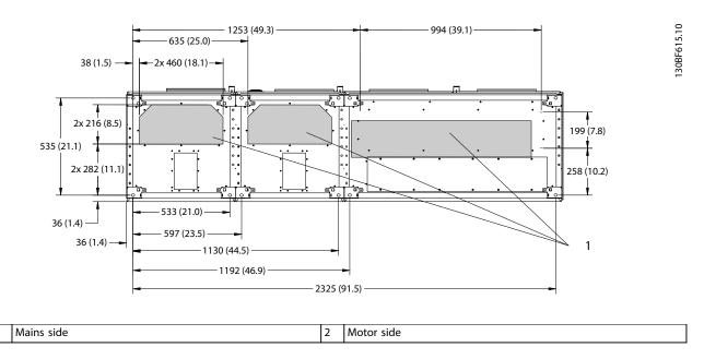
Figure 8.46 Gland Plate Dimensions for F4
