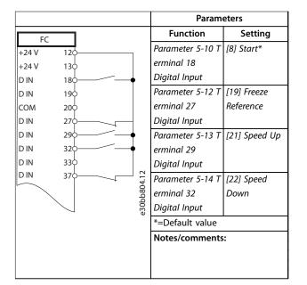
Table 12.10 Wiring Configuration for Speed Up/Speed Down
