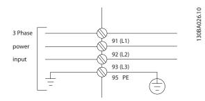
Figure 10.2 Connection of Mains, Enclosures E1-E2 and F1-F4
