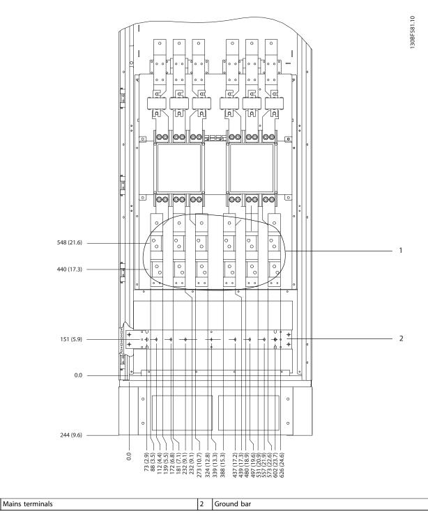
Figure 8.74 Terminal Dimensions for F11/F13 Options Cabinet, Front View
