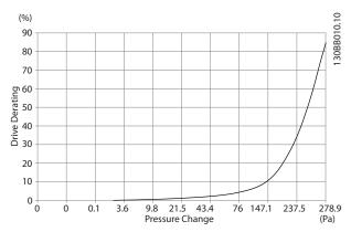
Figure 9.5 Derating vs. Pressure Change for E1–E2 Enclosures, 380–480 V Models: P315 and 525–690 V Models: P450–P500. Airflow: 650 cfm (1105 m<sup>3</sup>/h)
