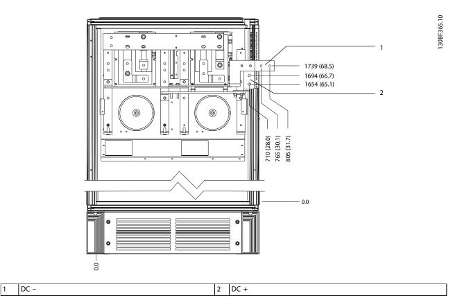
Figure 8.25 Terminal Dimensions for F1/F3 Regeneration Terminals, Front View
