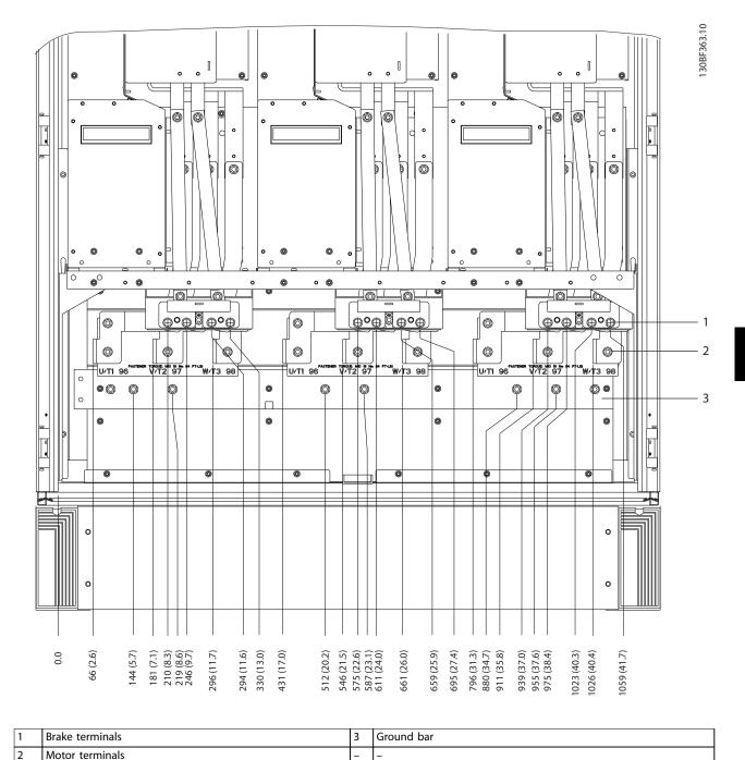
Figure 8.53 Terminal Dimensions for F2/F4 Inverter Cabinet, Front View
