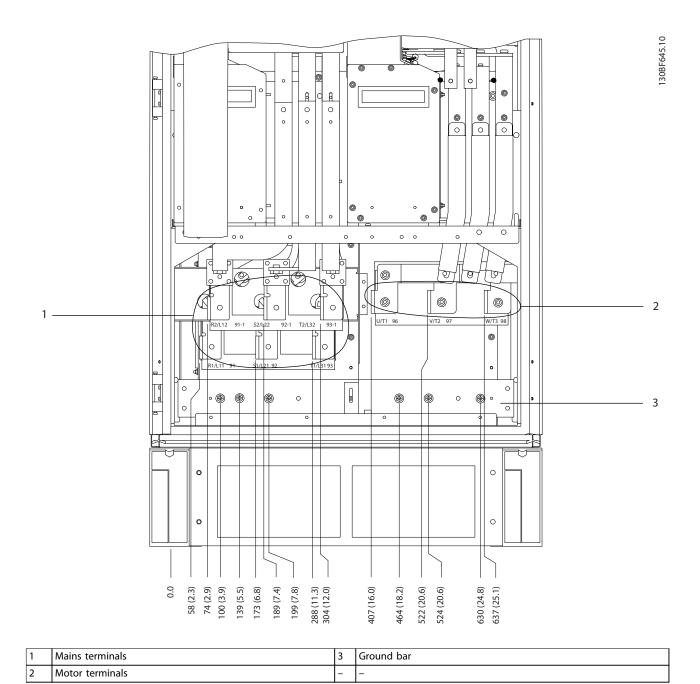
Figure 8.64 Terminal Dimensions for F8–F9 Rectifier/Inverter Cabinet, Front View
