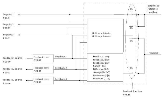
Figure 11.4 Block Diagram of Feedback Signal Processing
