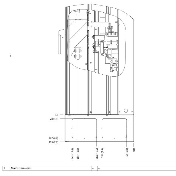
Figure 8.7 Terminal Dimensions for E1 with Disconnect (380-480/500 V Models: P315; 525-690 V Models: P355-P560), Side View
