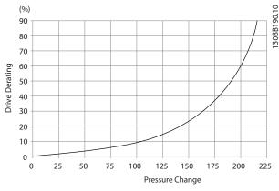
Figure 9.7 Derating vs. Pressure Change for Enclosures F1–F4. Airflow: 580 cfm (985 m<sup>3</sup>/h)
