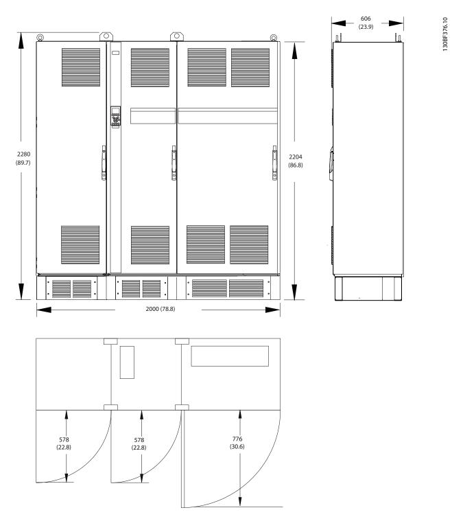
Figure 8.33 Front, Side, and Door Clearance Dimensions for F3
