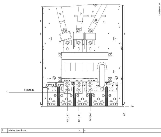
Figure 8.15 Terminal Dimensions for E2 with Disconnect (380-480/500 V Models: P315; 525-690 V Models: P355-P560), Front View
