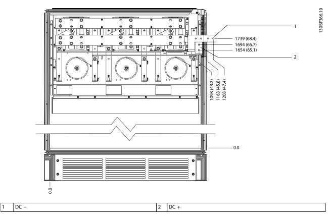
Figure 8.32 Terminal Dimensions for F2/F4 Regeneration Terminals, Front View
