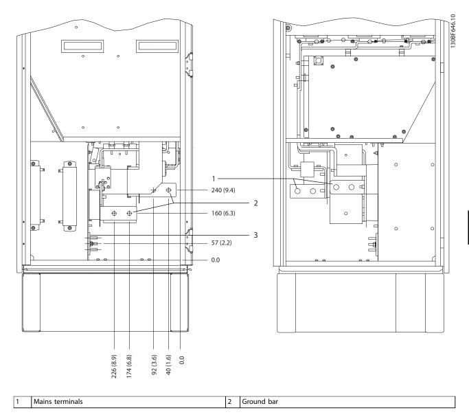
Figure 8.69 Terminal Dimensions for F10-F13 Rectifier Cabinet, Side View
