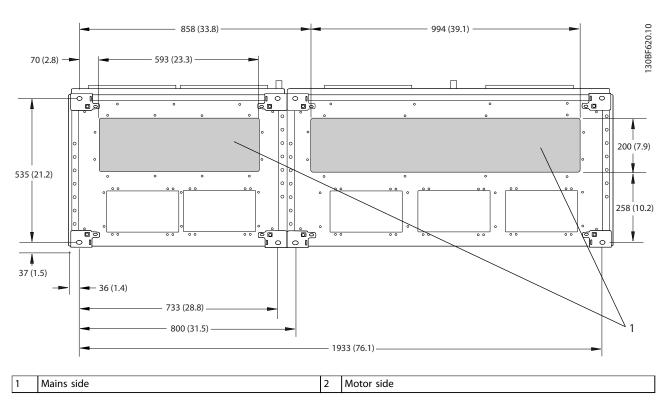
Figure 8.81 Gland Plate Dimensions for F12
