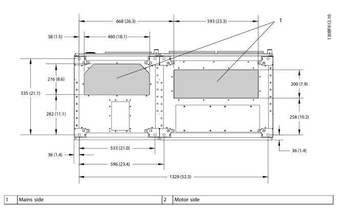
Figure 8.20 Gland Plate Dimensions for F1
