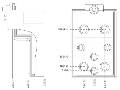
Figure 8.12 Detailed Terminal Dimensions for E1/E2
