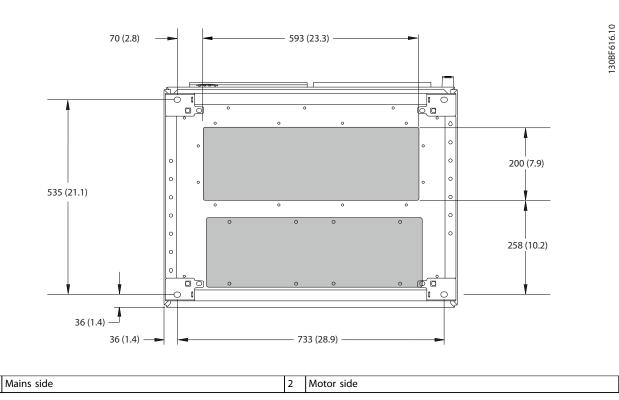
Figure 8.57 Gland Plate Dimensions for F8
