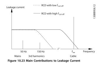
The amount of leakage current detected by the RCD depends on the cut-off frequency of the RCD.
