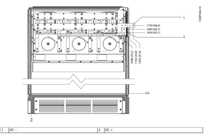
Figure 8.55 Terminal Dimensions for F2/F4 Regeneration Terminals, Front View
