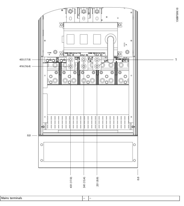
Figure 8.8 Terminal Dimensions for E1 with Disconnect (380-480/500 V Models: P355-P400), Front View
