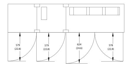
Figure 8.45 Front, Side, and Door Clearance Dimensions for F4
