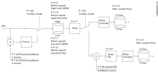
Figure 11.8 Control Structure in VVC<sup>+</sup> Open Loop and Closed-loop Configurations
