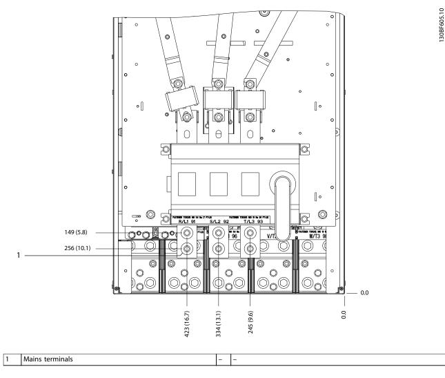
Figure 8.17 Terminal Dimensions for E2 with Disconnect (380–480/500 V Models: P355–P400), Front View
