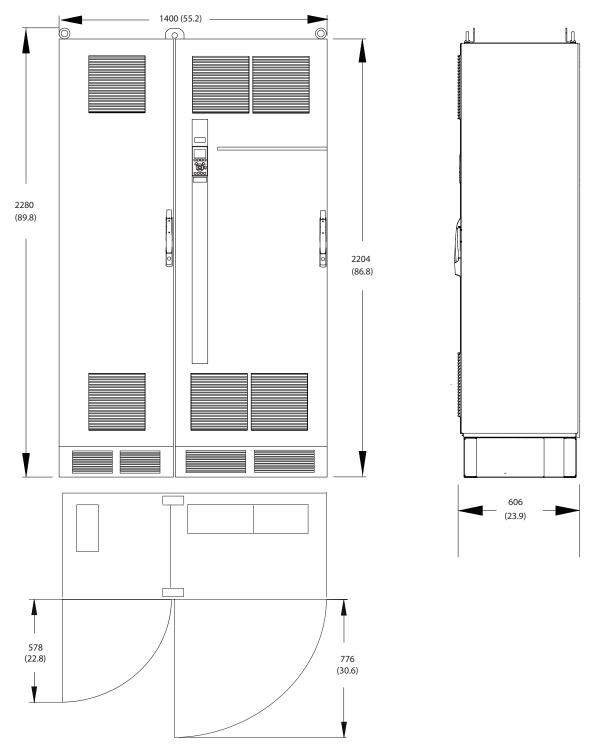
Figure 8.60 Front, Side, and Door Clearance Dimensions for F9
