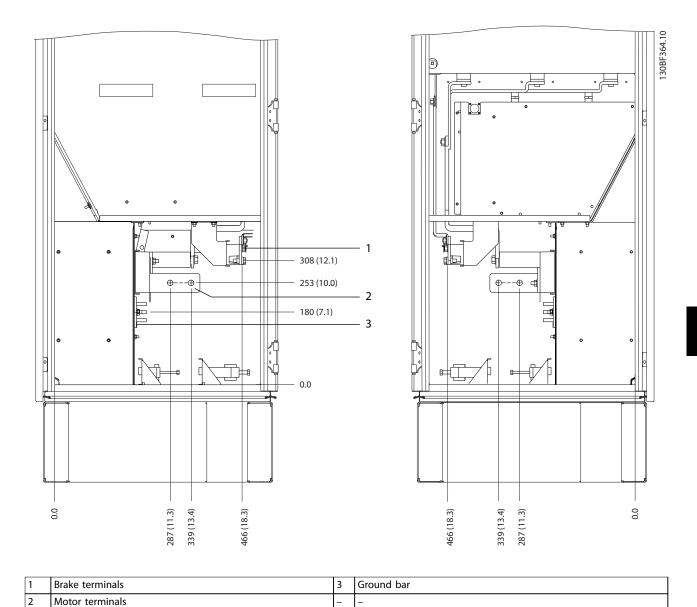
Figure 8.93 Terminal Dimensions for F12-F13 Inverter Cabinet, Side View
