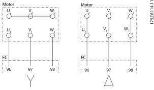
Figure 10.5 Motor Cable Connection
