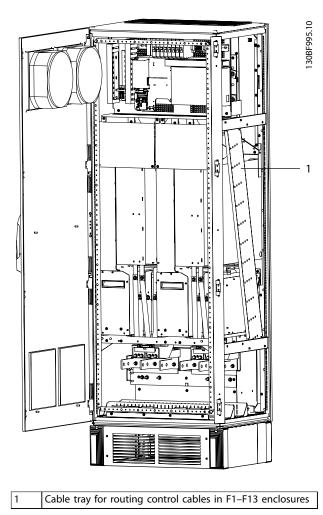
Figure 10.9 Control Card Wiring Path for the F1/F3. Control Card Wiring for the F2/F4 and F8–F13 Use the Same Path
