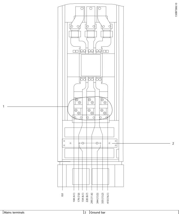
Figure 8.37 Terminal Dimensions for F3–F4 Options Cabinet with Circuit Breaker/Molded Case Switch, Front View
