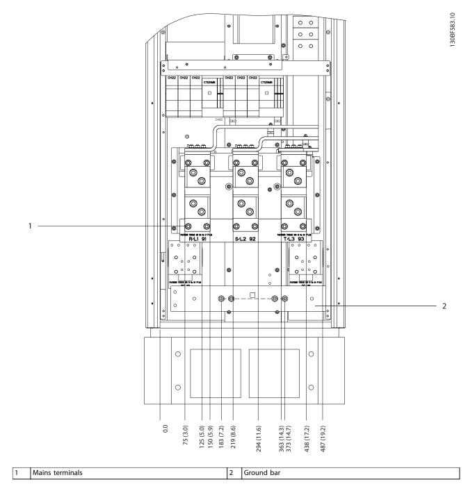
Figure 8.28 Terminal Dimensions for F1-F4 Rectifier Cabinet, Front View
