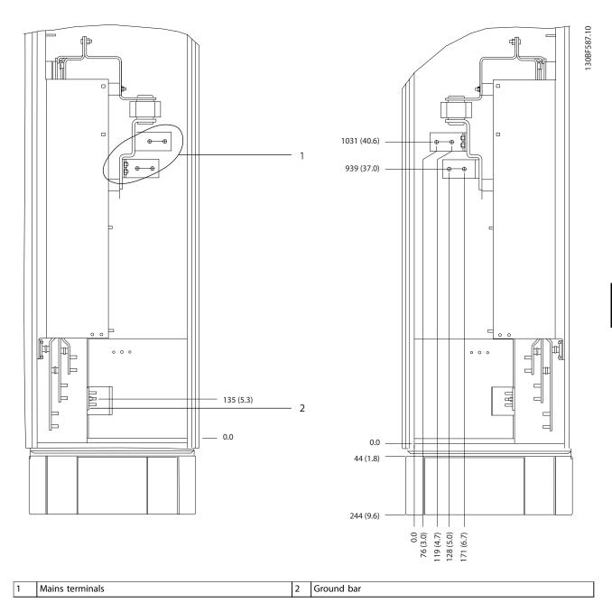
Figure 8.63 Terminal Dimensions for F9 Options Cabinet, Side View
