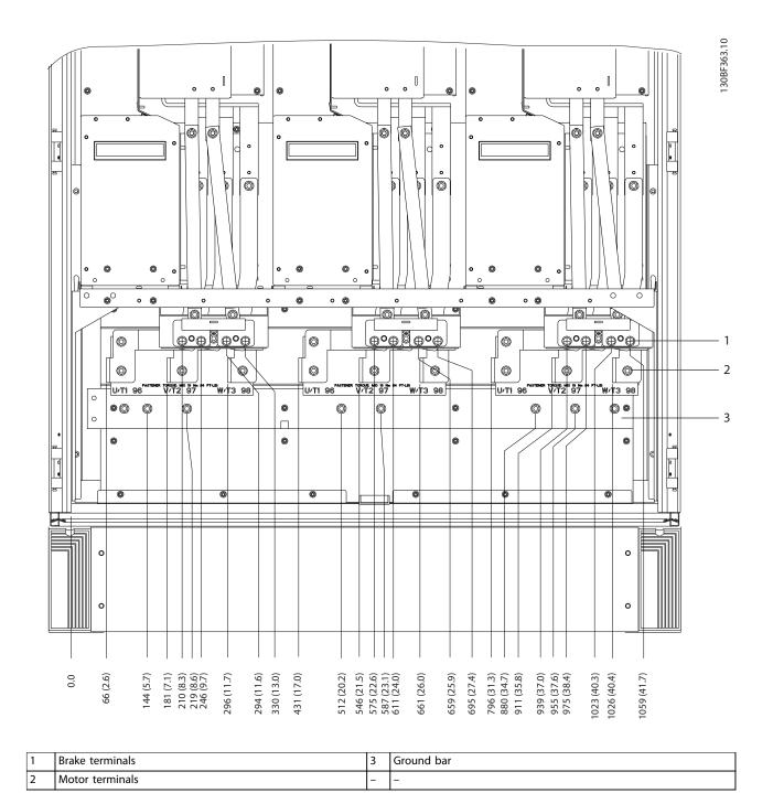
Figure 8.30 Terminal Dimensions for F2/F4 Inverter Cabinet, Front View
