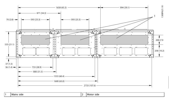
Figure 8.87 Gland Plate Dimensions for F13
