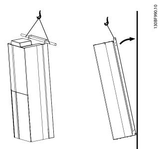
Figure 9.1 Recommended Lifting Method for E1-E2 Enclosures
