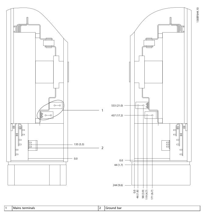
Figure 8.50 Terminal Dimensions for F3-F4 Options Cabinet with Circuit Breaker/Molded Case Switch, Side View
