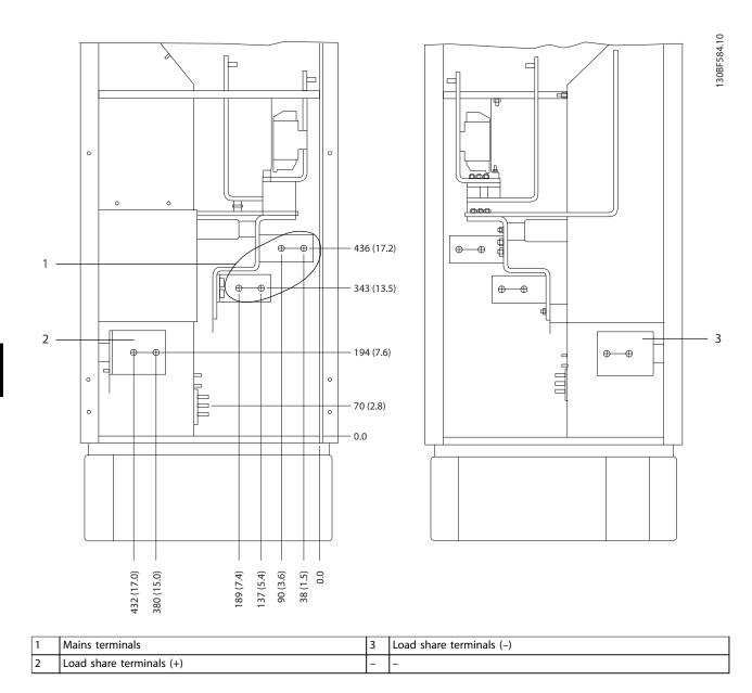
Figure 8.22 Terminal Dimensions for F1-F2 Rectifier Cabinet, Side View
