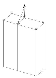
Figure 9.2 Recommended Lifting Method for F1/F2/F9/F10 Enclosures
