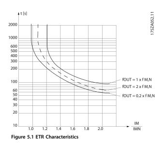
The X-axis shows the ratio between  $I_{motor}$  and  $I_{motor}$  nominal. The Y-axis shows the time in seconds before the ETR cuts off and trips the drive. The curves show the characteristic nominal speed, at twice the nominal speed and at 0.2 x the nominal speed.
