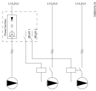
Figure 12.7 Fixed Variable Speed Pump Wiring Diagram
