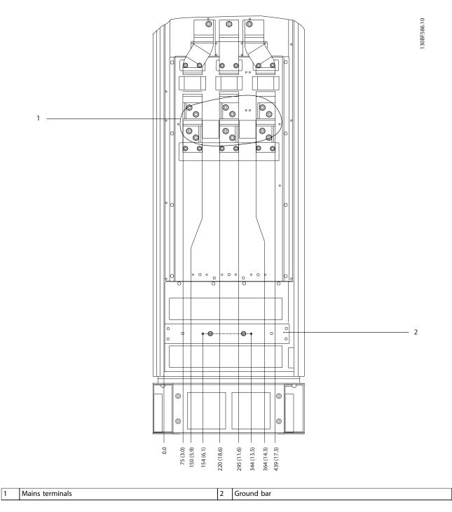
Figure 8.35 Terminal Dimensions for F3-F4 Options Cabinet, Front View
