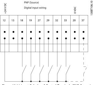
Figure 10.14 Input Polarity of Control Terminals (PNP Source)
