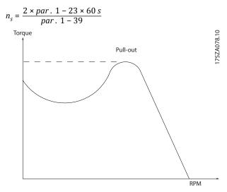
Figure 14.1 Break-away Torque Chart
