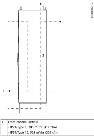
2 Back-channel airflow, 985 m<sup>3</sup>/hr (580 cfm)
