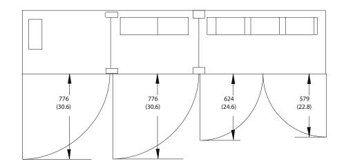
Figure 8.86 Front, Side, and Door Clearance Dimensions for F13
