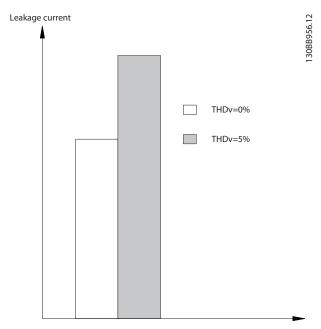
Figure 10.22 Line Distortion Influences Leakage Current
