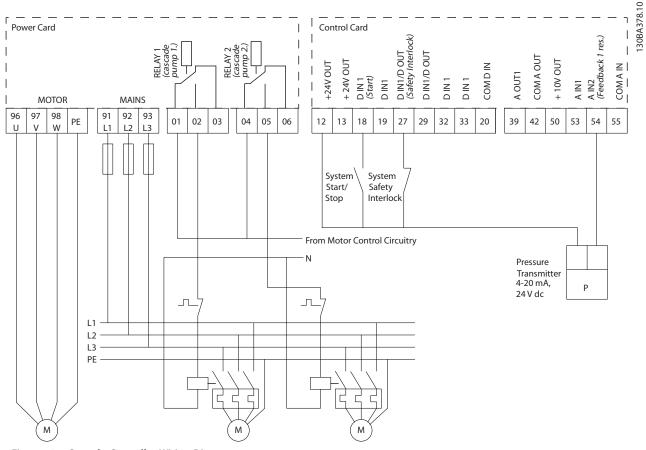
Figure 12.4 Cascade Controller Wiring Diagram
