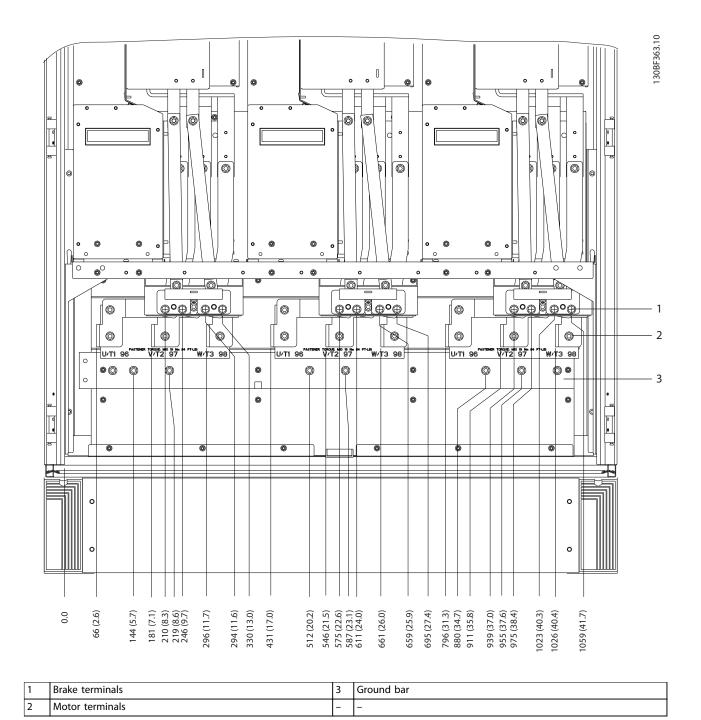
Figure 8.92 Terminal Dimensions for F12-F13 Inverter Cabinet, Front View
