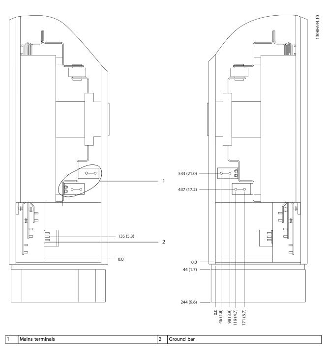
Figure 8.39 Terminal Dimensions for F3-F4 Options Cabinet with Circuit Breaker/Molded Case Switch (380-480/500 V Models: P500-P630; 525-690 V Models: P800), Side View
