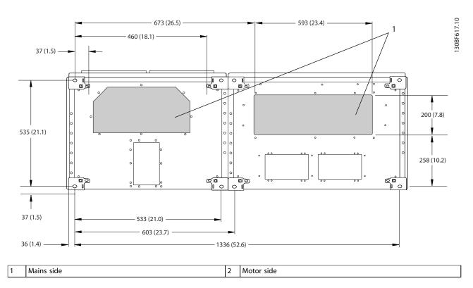
Figure 8.61 Gland Plate Dimensions for F9
