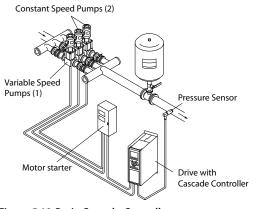
Figure 5.10 Basic Cascade Controller
