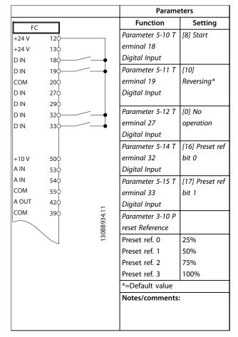
Table 12.7 Wiring Configuration for Start/Stop with Reversing and 4 Preset Speeds
