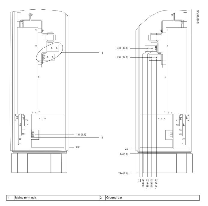
Figure 8.36 Terminal Dimensions for F3-F4 Options Cabinet, Side View
