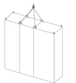
Figure 9.3 Recommended Lifting Method for F3/F4/F11/F12/F13 Enclosures
