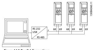
Figure 14.2 Parallel Connections
