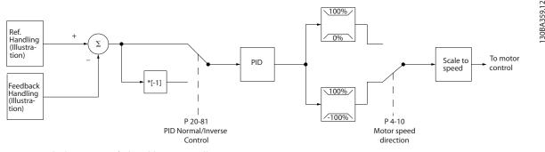
Figure 11.7 Block Diagram of Closed-loop Controller
