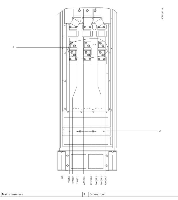
Figure 8.47 Terminal Dimensions for F3-F4 Options Cabinet, Front View
