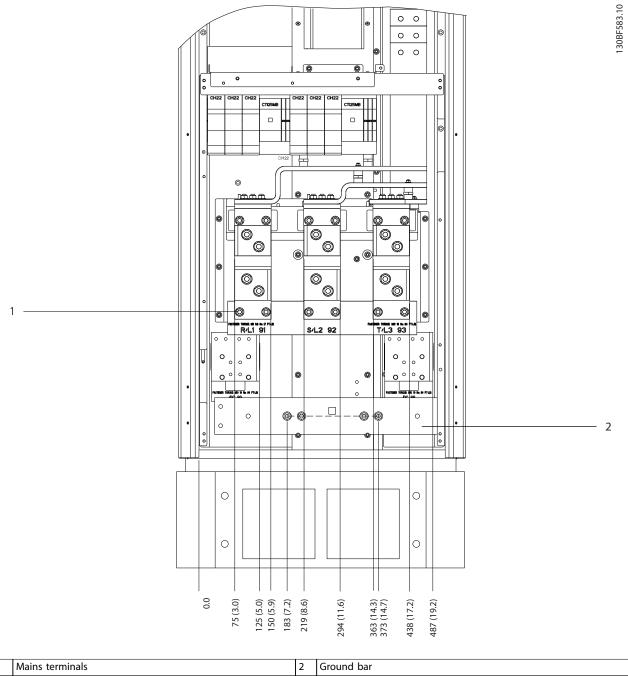
Figure 8.21 Terminal Dimensions for F1-F4 Rectifier Cabinet, Front View
