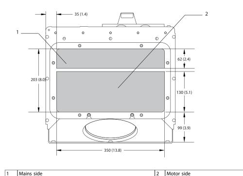
Figure 8.11 Gland Plate Dimensions for E1/E2
