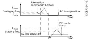
Figure 5.11 Lead Pump Alternation
