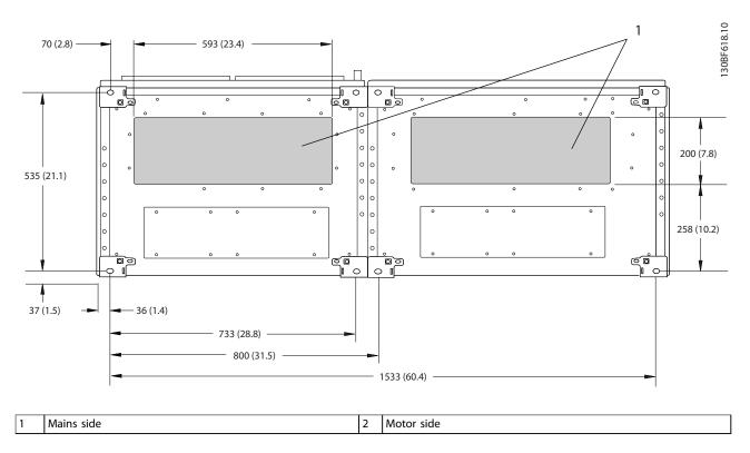
Figure 8.67 Gland Plate Dimensions for F10
