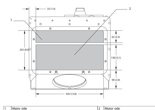
Figure 8.2 Gland Plate Dimensions for E1/E2
