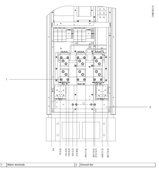
Figure 8.51 Terminal Dimensions for F1-F4 Rectifier Cabinet, Front View
