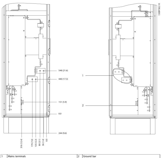
Figure 8.75 Terminal Dimensions for F11/F13 Options Cabinet, Side View
