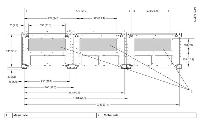
Figure 8.73 Gland Plate Dimensions for F11
