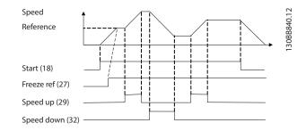
Figure 12.3 Speed Up/Speed Down
