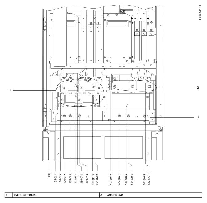
Figure 8.90 Terminal Dimensions for F10-F13 Rectifier Cabinet, Front View
