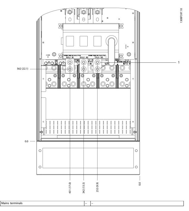
Figure 8.6 Terminal Dimensions for E1 with Disconnect (380-480/500 V Models: P315; 525-690 V Models: P355-P560), Front View
