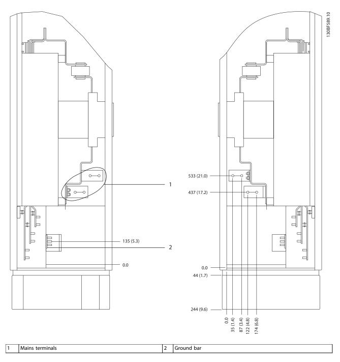
Figure 8.38 Terminal Dimensions for F3–F4 Options Cabinet with Circuit Breaker/Molded Case Switch (380–480/500 V Models: P450; 525–690 V Models: P630–P710), Side View
