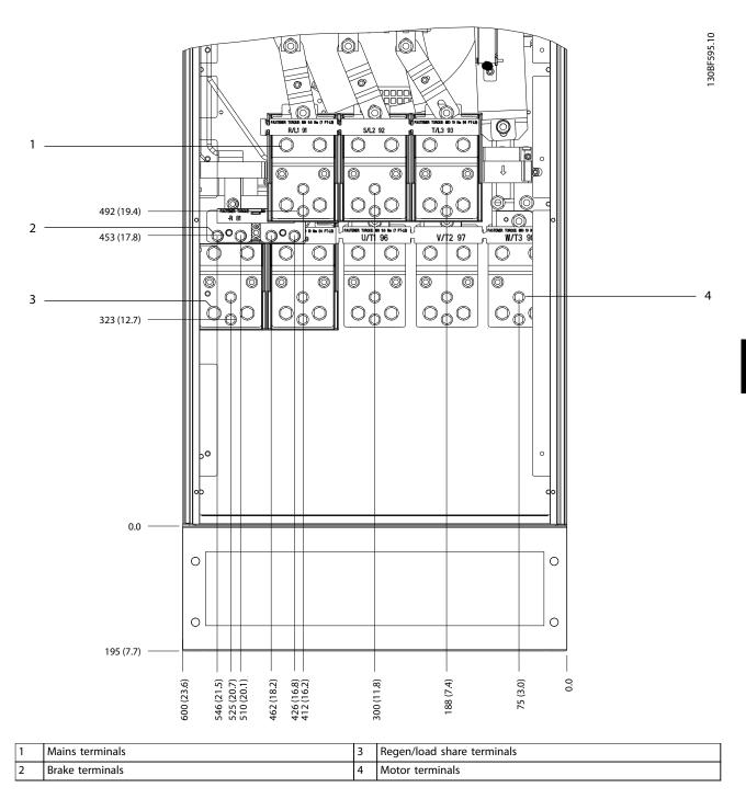
Figure 8.4 Terminal Dimensions for E1, Front View
