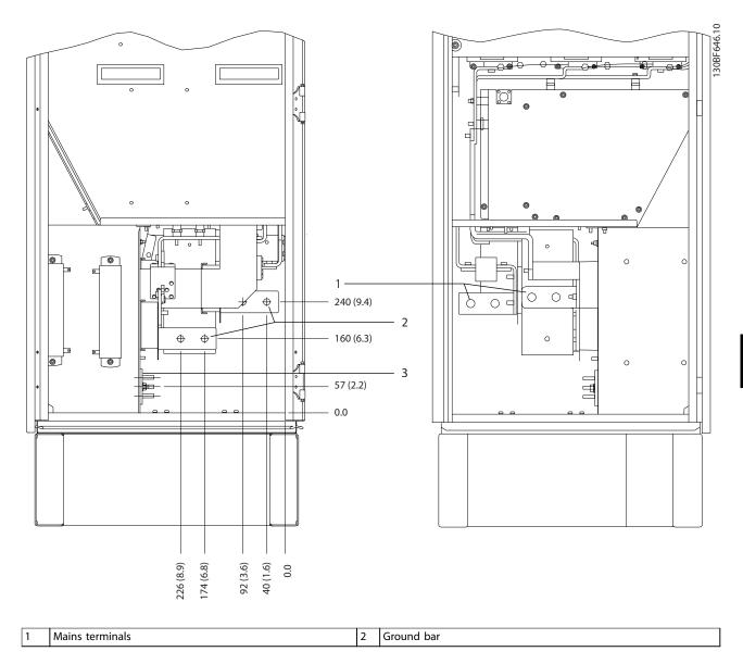
Figure 8.77 Terminal Dimensions for F10-F13 Rectifier Cabinet, Side View
