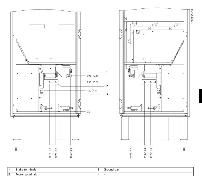
Figure 8.31 Terminal Dimensions for F2/F4 Inverter Cabinet, Side View
