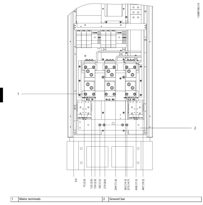
Figure 8.40 Terminal Dimensions for F1-F4 Rectifier Cabinet, Front View
