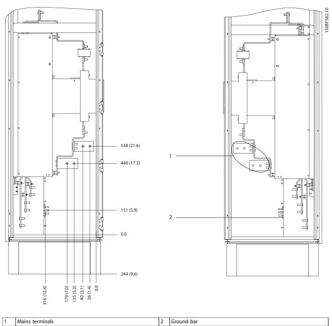
Figure 8.89 Terminal Dimensions for F11/F13 Options Cabinet, Side View
