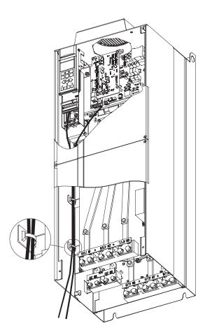
Figure 10.8 Control Card Wiring Path for the E1 and E2 Enclosures
