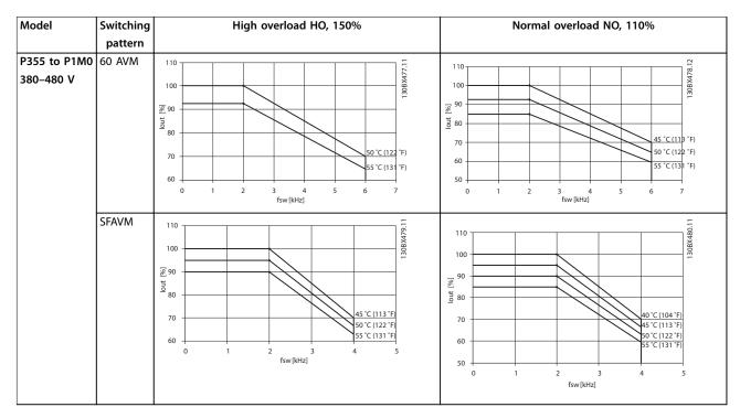
Table 9.4 Ambient Temperature Derating Tables for E1–E2, F1–F4, and F8–F13 Enclosures, 380–480 V
