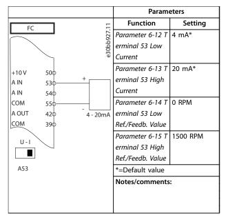
Table 12.4 Wiring Configuration for Analog Speed Reference (Current)
