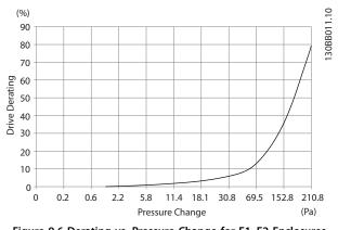
Figure 9.6 Derating vs. Pressure Change for E1–E2 Enclosures, 380–480 V Models: P355–P450 and 525–690 V Models: P560–P630. Airflow: 850 cfm (1445  $m^3/h$ )
