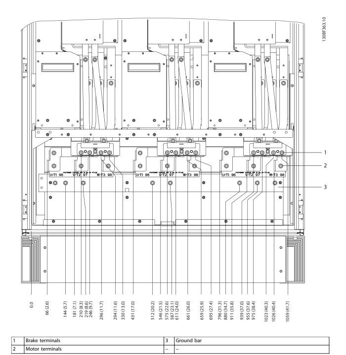
Figure 8.84 Terminal Dimensions for F12-F13 Inverter Cabinet, Front View
