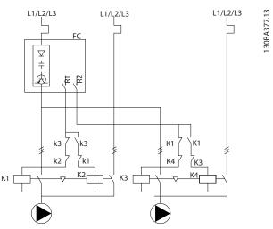
Figure 12.8 Lead Pump Alternation Wiring Diagram.
