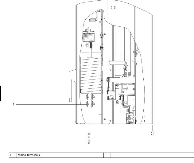
Figure 8.16 Terminal Dimensions for E2 with Disconnect (380-480/500 V Models: P315; 525-690 V Models: P355-P560), Side View
