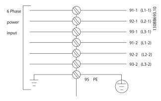
Figure 10.3 Connection of Mains, Enclosures F8–F13
