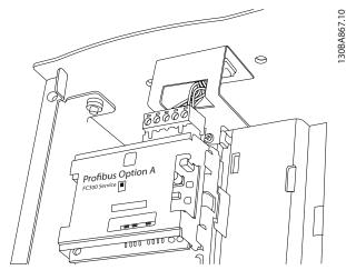
Figure 10.10 Top Connection for Fieldbus
