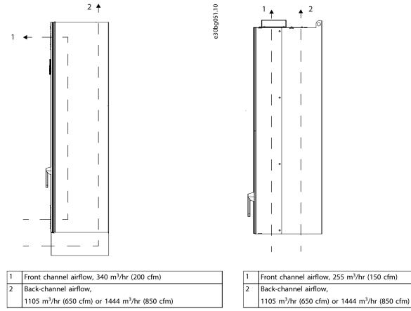
Figure 7.2 Airflow for Enclosure E1
