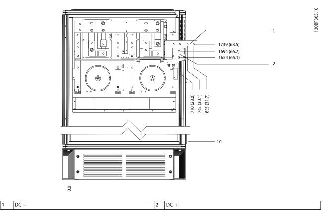
Figure 8.44 Terminal Dimensions for F1/F3 Regeneration Terminals, Front View
