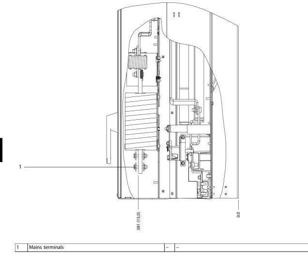
Figure 8.18 Terminal Dimensions for E2 with Disconnect (380-480/500 V Models: P355-P400), Side View
