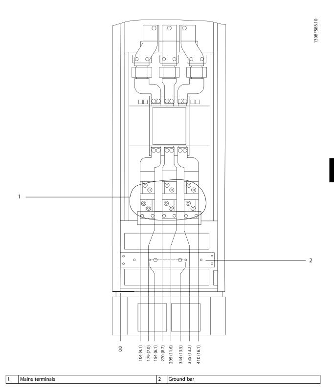
Figure 8.49 Terminal Dimensions for F3–F4 Options Cabinet with Circuit Breaker/Molded Case Switch, Front View
