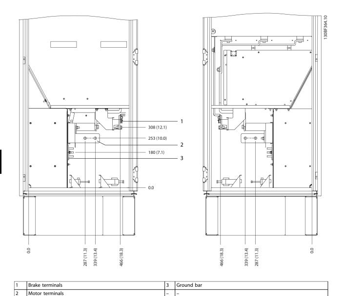
Figure 8.54 Terminal Dimensions for F2/F4 Inverter Cabinet, Side View
