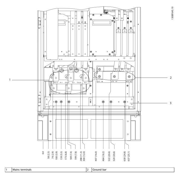
Figure 8.82 Terminal Dimensions for F10-F13 Rectifier Cabinet, Front View
