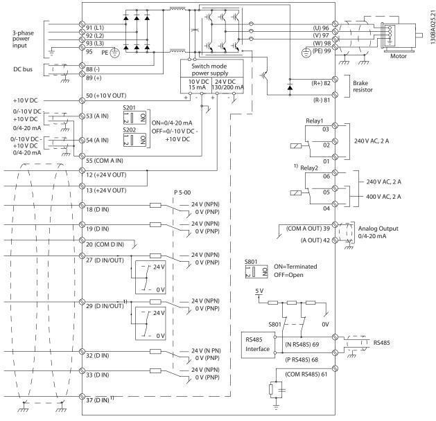
Figure 10.1 Basic Wiring Schematic
