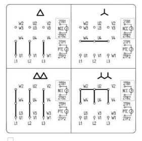
Figure 16: Terminal board connection - motor series 11N, 11P and 22P
