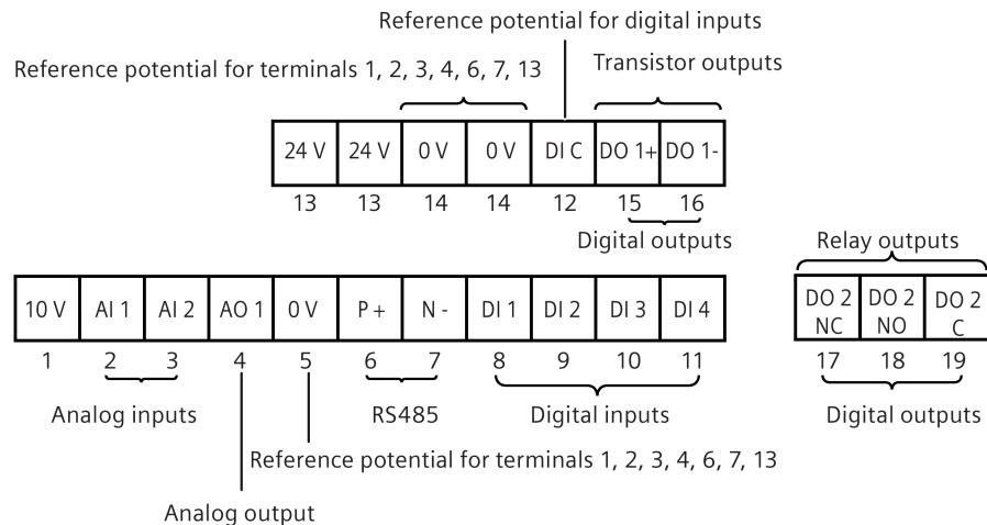
**User terminals for FSA to FSE:**
