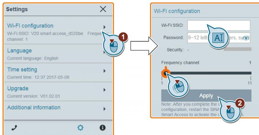
Note that the new Wi-Fi configuration takes effect only after the SINAMICS V20 Smart Access restarts.
