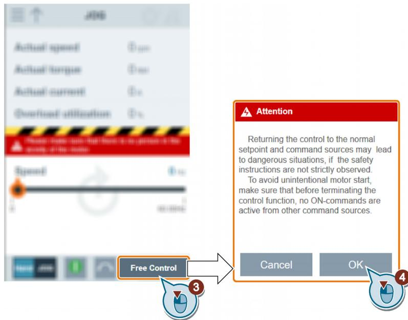
Note that before relinquishing control, make sure that there is no converter output and the motor has come to a standstill. If the motor is still running, the following message appears:
