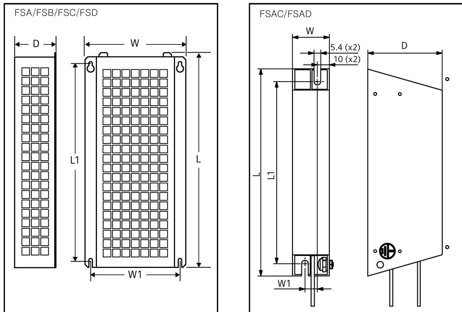
**For single phase AC 230 V converters FSAA to FSAB and three phase AC 400 V converter FSE**
