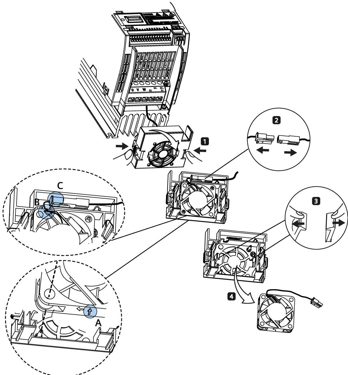
Replacing the fan(s) from FSB, FSC or FSD
