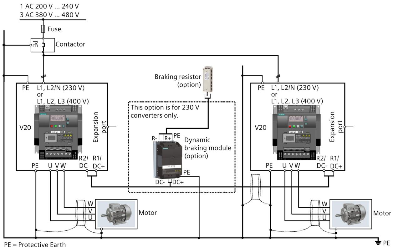
See Section "Terminal description (Page 45)" for the recommended cable cross-sections and screw tightening torques.
