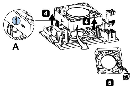
Replacing the fan from FSAD
