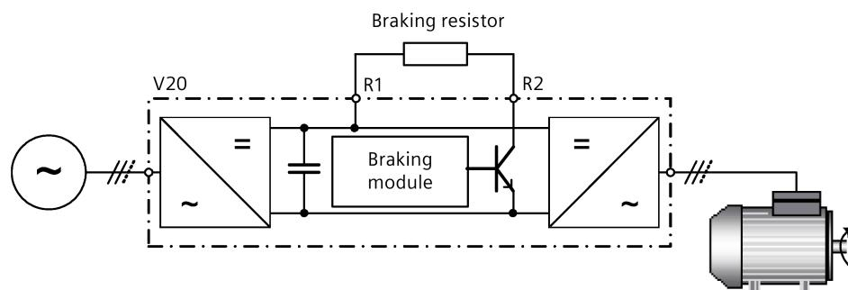
The continuous power  $P_{DB}$  and the duty cycle for the braking resistor can be modified using the dynamic braking module (for single phase AC 230 V converters) or parameter P1237 (for three phase AC 400 V converters).
