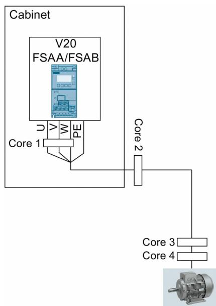
For 230 V filtered and unfiltered frame size AC converters with the maximum motor cable length of 10 m:
