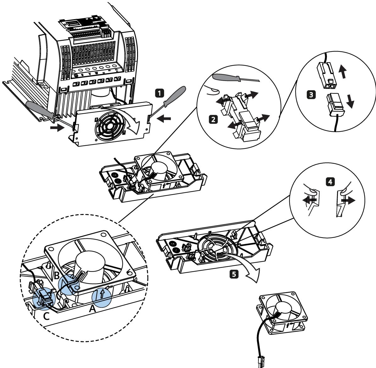
Replacing the fans from FSE
