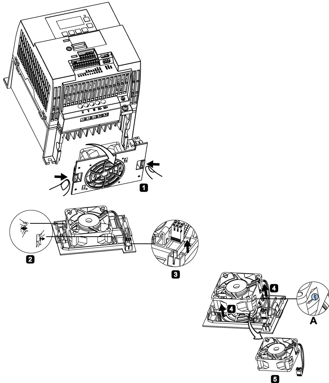
Replacing the fan from FSA
