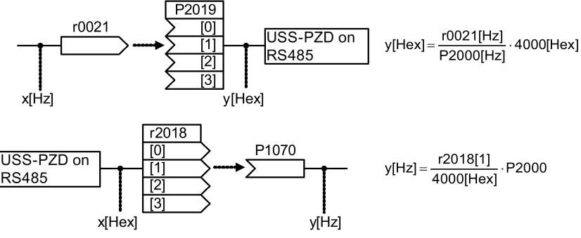
$y[\text{Hex}] = \frac{r0021[\text{Hz}]}{P2000[\text{Hz}]} \cdot 4000[\text{Hex}]$ $y[\text{Hz}] = \frac{r2018[1]}{4000[\text{Hex}]} \cdot P2000$                                                                     |               |                 |                |         |          |           |            |  |
