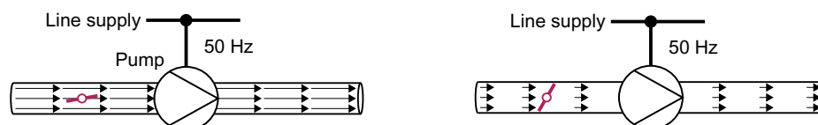
Figure 8-82 Flow control with pump and throttle connected to a 50 Hz line supply
